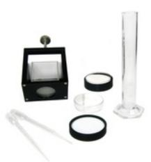
Use the F-750 to measure quality indicators in liquids, powders, and irregular solids with the F-750LK Liquids and Powders Kit. The table-mount Liquids Kit enables the operator to measure liquids in the included high-quality glass cuvettes (2 x 1 cm path length, 1 x 5 cm path length) which fit down inside the adjustable holder. For powders, irregular solids, and viscous fluids, use the custom-built petri dish holder to take measurements in one of the 5 included plastic petri dishes.
