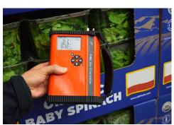
The F-940 Store It! Gas Analyzer provides rapid and precise measurements of ethylene, CO<sub>2</sub> and O<sub>2</sub>. The Store It! was designed for Quality Assurance staff to increase shelf-life and prevent spoilage by monitoring ripening gases throughout the storage process.
