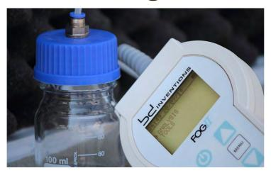
On the go determination of the total inorganic carbon as equivalent calcium carbonate with **GPS** content technology
