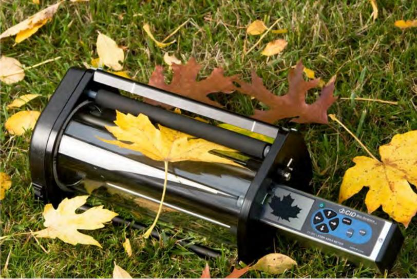
Measure large numbers of detached leaves rapidly by inserting the CI-203 Handheld Laser Leaf Area Meter into the CI-203CA Conveyor Attachment.
