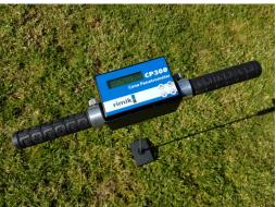
This instrument can be user configured to operate in metric or imperial mode. The menu structure also allows the user to preselect any of four (4) depth intervals and to preselect any of six (6) cone sizes. Data can also be "Grouped" by nominating a group size (up to 500) prior to taking any set of insertions. The groups can be individually named.
