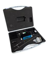
The CP300 cone penetrometer is used to measure soil density and hardness where a research level study of the data is required. It measures and records cone index values up to 9800KPa based on the load required to force a cone through the soil. The instrument will record profile data to a maximum depth of 750mm at increments of 10 - 25mm. The instrument conforms to ASAE S313.3 feb99.
